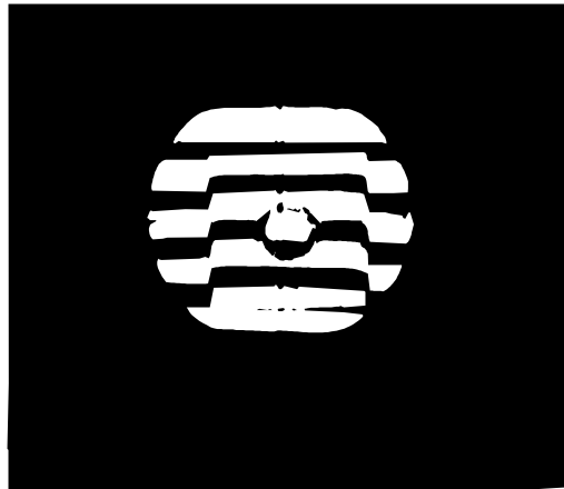
Fig. 6.2 Observed fringe pattern for a gauge block wrung to a platen.
