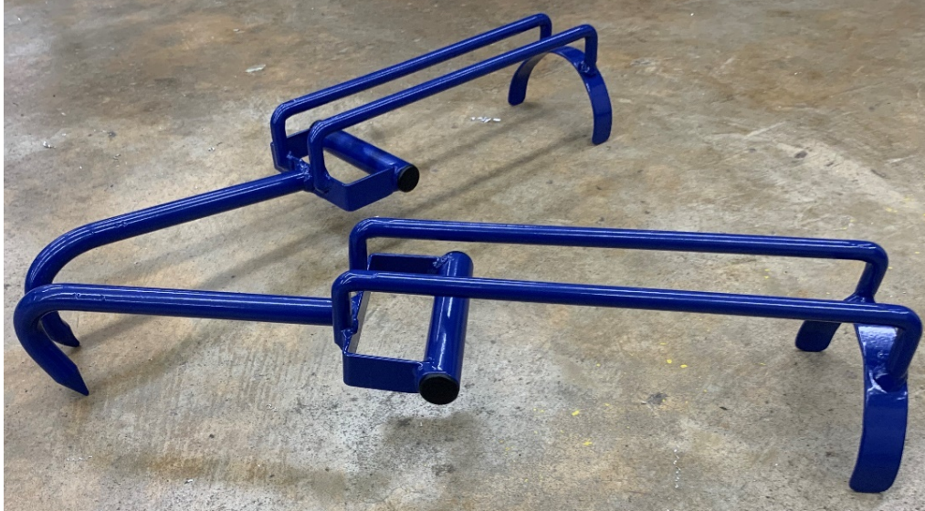
Figure 9 Completed Hay Hooks
