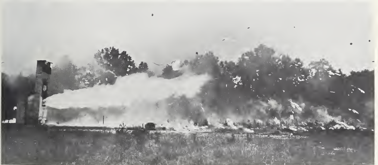
FIGURE 2.3. Explosion of cellulose nitrate film from decomposition in storage.
