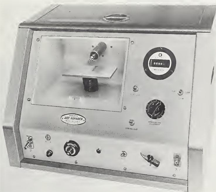
FIGURE 3.1. Roberts jet abrader for measuring abrasion resistance as described in Fed. Test Method Std. No. 141a, Test Method 6193. (Photo courtesy of Kameron Instruments.)
