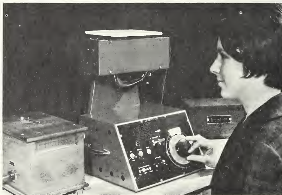
FIGURE 6.1. Glossmeter measures specular reflectance of surfaces and coatings as described in ASTM Method D 523-66T.
