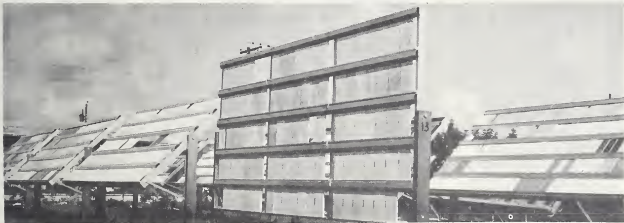
FIGURE 8.2. Modern outdoor exposure racks can be set for any angle in a single longitudinal plane. Hinged cross bars are adjustable to retain specimens of different lengths.
