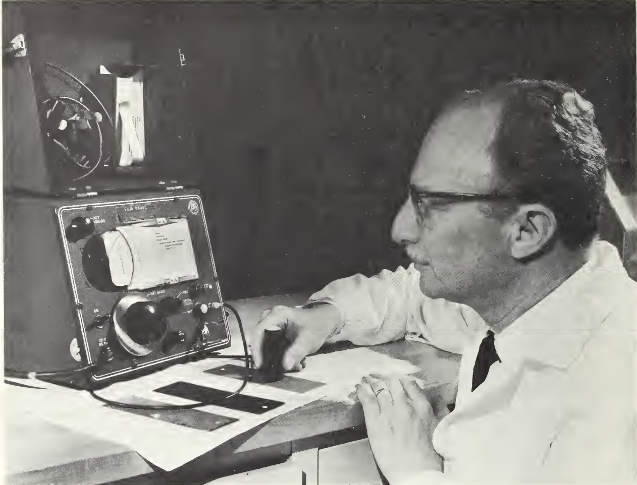
FIGURE 7.1. Eddy-current thickness gage for nondestructive measurement of thickness of nonconductive coatings on metal substrates, as described in ASTM Method D 1400-67T. (See text, p. 138.)
