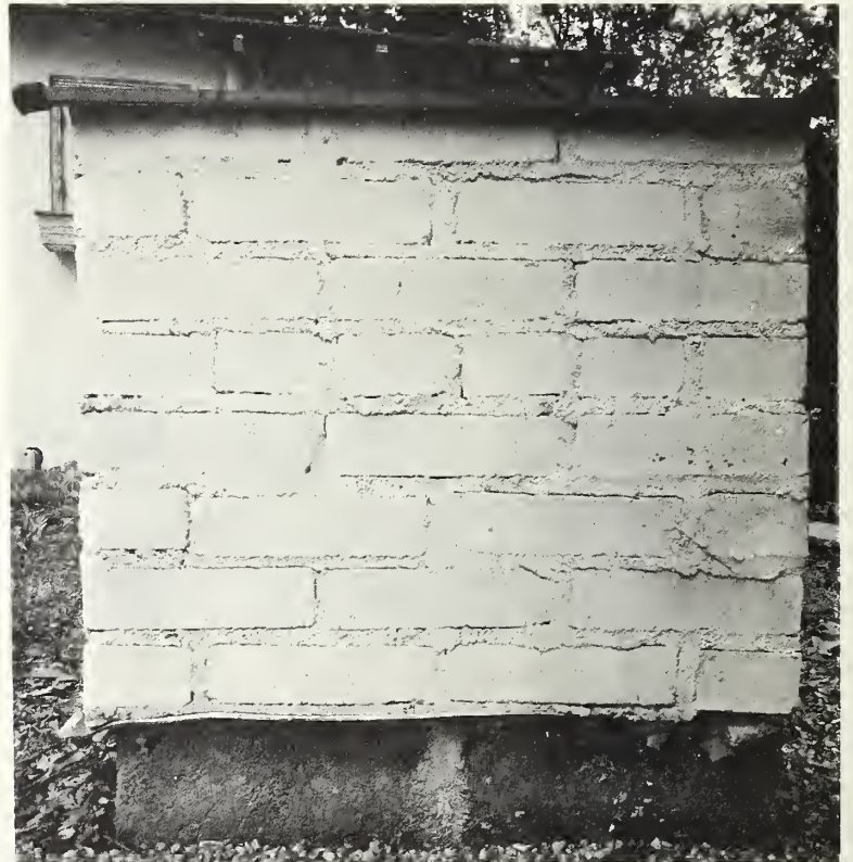
FIGURE 8.4. A typical masonry-wall specimen used to conduct paint exposure tests.
