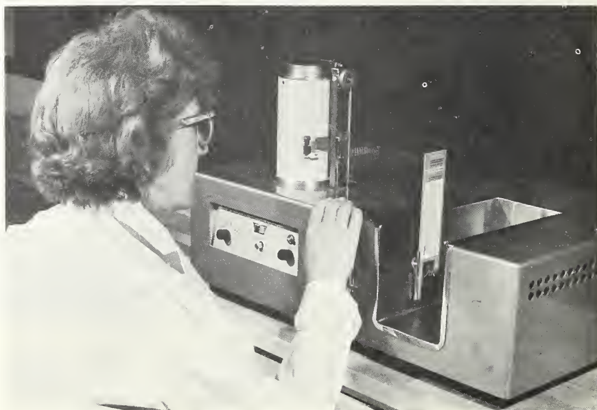
FIGURE 3.3. Infrared spectrophotometer is used to identify binders, solvents, and pigments in organic coatings.
